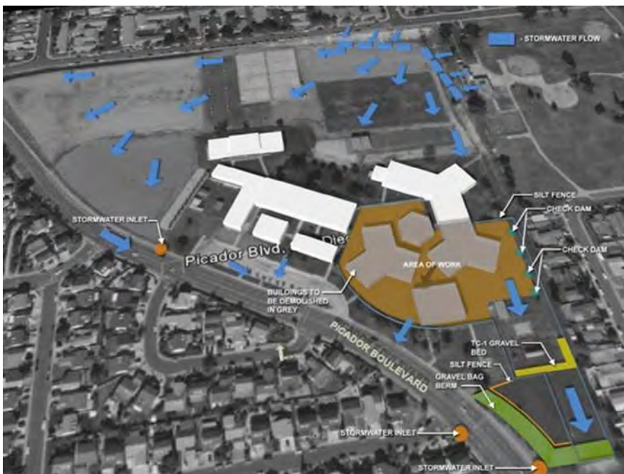
Figure 3.9 Stormwater runoff prevention plan
