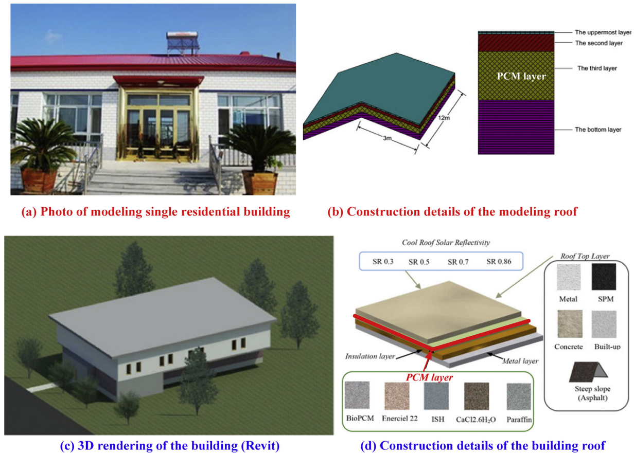
Fig. 7. Prototype of modeling building and construction details of its roof [26,27].
