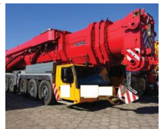
2010 Liebherr LTM1500-8.1 50M Boom; 21M-91M Luffing Jib; 14M-63M Fixed Lattice Jib; Y-Guide Superlift; Liebherr Diesel Engines; 3 Winches; 445.95R25 Tires; 16x8x12 Drive; 165 Ton Counterweight; 4,600 hours / 48,000 Km
