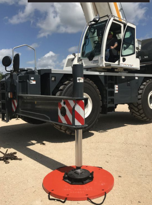
COMPOSITE OUTRIGGER PADS AVAILABLE IN ANY CUSTOM SIZE & SHAPE
