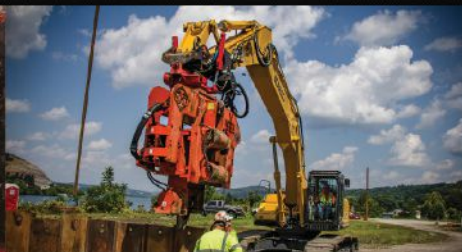
V-5 Esc Vibratory Pile Driver • 53 Tons of Driving Force
