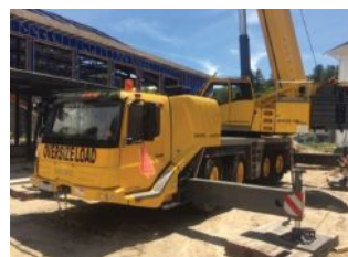
2013 Grove GMK4115L 197' 7-section Full Power Boom; Single Boom Lift Cylinder; 33'-56' Hydraulic Luffing Jib; 2 Winches; 7,825 Km; 8,253 hours – Upper
