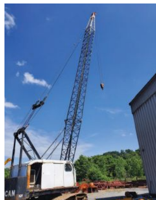
1967 American 5299 100' Boom; GM4-71 w/ Twin Disc Torque Converter; 3rd Drum; Control Load Lowering; 36" Shoes; Block; "As Is"
