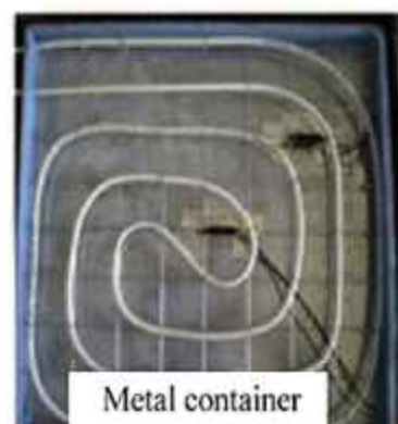
(b) Floor specimen placed and tested inside a small adiabatic room
