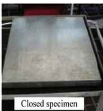
(b) Floor specimen placed and tested inside a small adiabatic room
